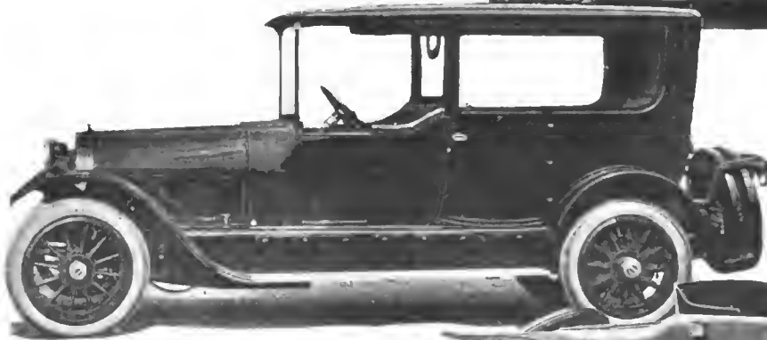
A permanent top product by Locomobile which may be quickly converted into an open body by lowering the windows
